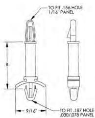
Micro Plastics' Circuit Board Supports eliminate screws, nuts, and lockwashers in mounting printed circuit
