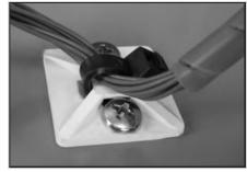
Cradle Mounts are used in applications where a low profile is necessary. Each mount offers a four way entry and is secured with either a screw or adhesive backing. 23TA00420 is secured with a #2 - #4 or #6 screw, 23TA00495 uses #6 Flat Head Screw.
