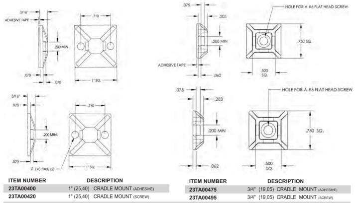
**NOTE**: the adhesive mounts have an acrylic foam backing that should be used on a smooth, clean, dry surface.
