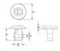
• PANEL HOLE DIAMETER .250 MAXIMUM PANEL THICKNESS .125
