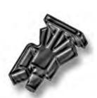
Heavy duty nylon 6/6 support snaps into P.C. board from bottom. Locking arm clips to the side of the P.C. board making for easy removal and replacement of P.C. boards. Support does not rotate in chassis or positioning holes. Board clearance may vary depending on chassis thickness. Parts are molded in black nylon.
