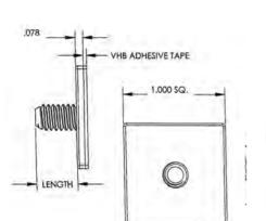
dry, and free of contamination. Firm pressure must be applied to increase the cold flow and contact of the adhesive with the substrate. Parts can be purchased without VHB adhesive foam. just add WOAF to the end of part number.
