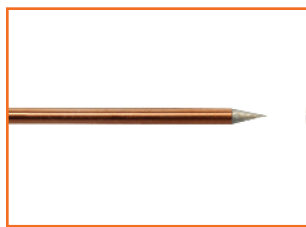
1. A sharpened dowel pin is selected—slightly smaller than the wire diameter
