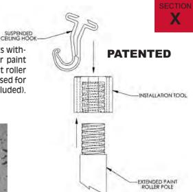
Hex shaped area is designed to fit a metric M6 hex nut or M6 hex head machine screw. **Note:** Insert nut or screw into installation tool before attaching to extension pole.
